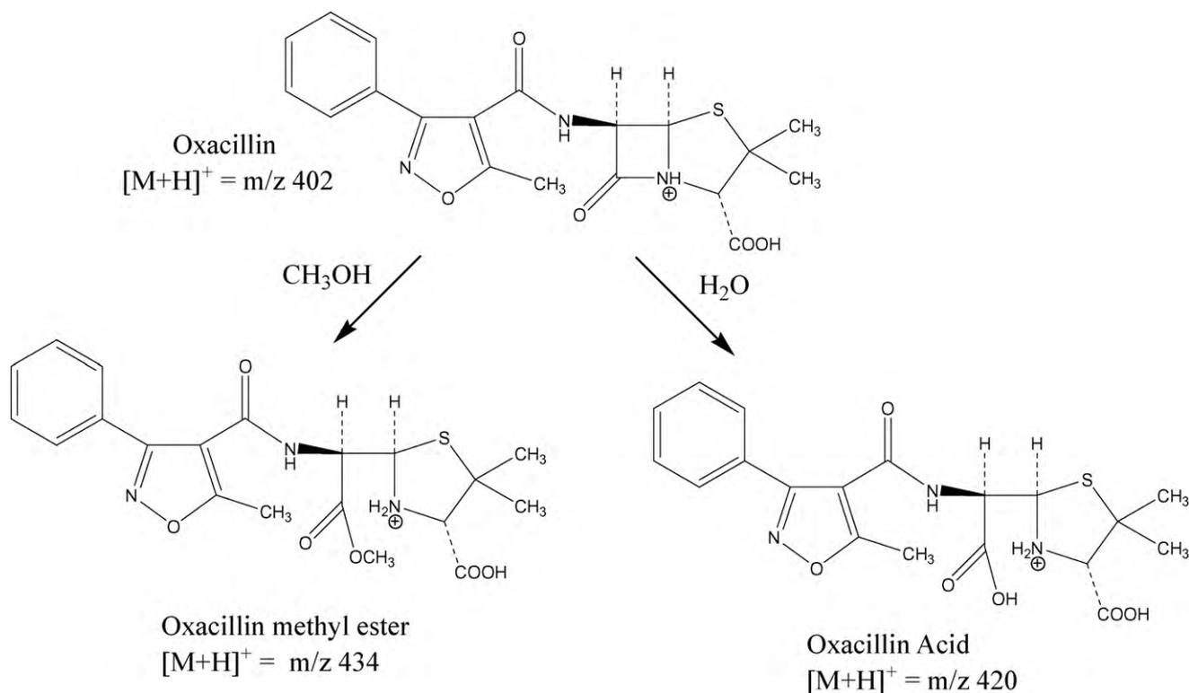
Fig. 2. Methanolysis and hydrolysis degradation products of oxacillin.
