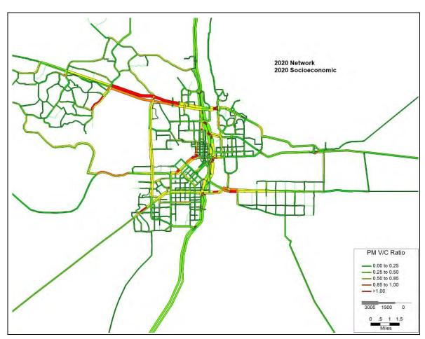
Figure 6.1: 2020 Base Year Scenario - PM Peak Volume to Capacity Ratio
