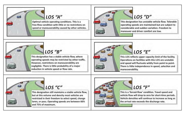
Figure 10.1: Highway Capacity Manual Level of Service (LOS)
