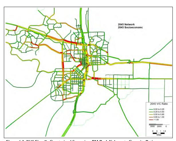
Figure 6.3: 2045 Fiscally Constrained Scenario – PM Peak Volume to Capacity Ratio
